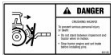
B. DANGER - Crushing Hazard Sign Number 461138
