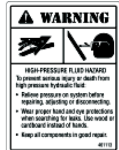
B. WARNING - High pressure Fluid Hazard Sign Number 461113
