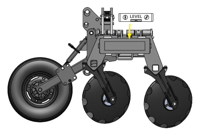
Tipping the machine front to back can be used to change the shape of the beds, by increasing or decreasing depth of the rear blades.
