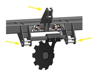
2. Once removed, the remaining pins are set to run the implement with a Category 3 hitch.
