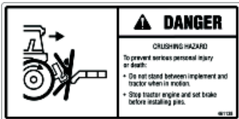
C. DANGER - Crushing Hazard Sign Number 461138
