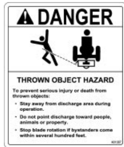
G. DANGER - Thrown Object Hazard. Sign Number 461087
